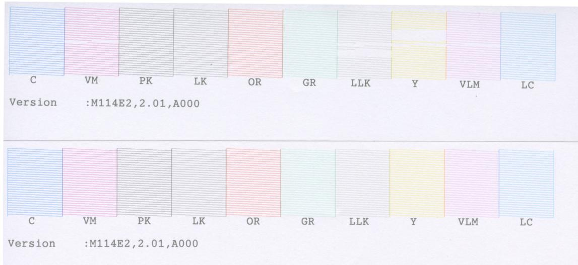
Notice the gaps in parts of the test sheet. These are print heads that need to be cleaned. Again, these are cleaned automatically when using **Auto**.
