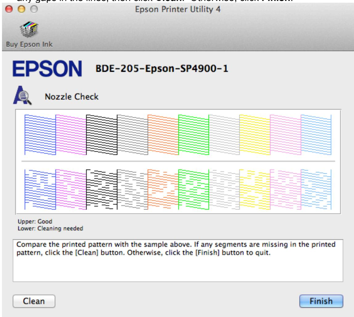
9. For **Auto**, simply click **Auto** and it will print out a test sheet while cleaning the print heads at the same time. This will always take longer than print, regardless of the heads are clean or not. A typical test sheet using **Auto** may look like this:
