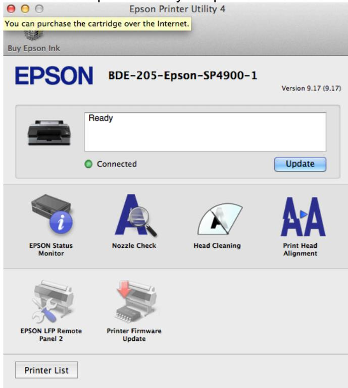
6. There are two ways to perform a Nozzle Check: **Print** and **Auto**. **Print** will simply print out a test sheet. **Auto** will run a print head cleaning at the same time.
