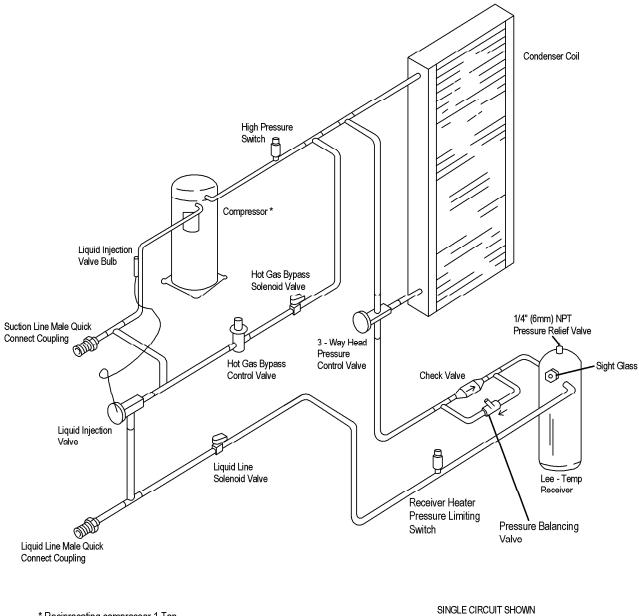
\* Reciprocating compressor 1 Ton. Scroll compressor 1 1/2 - 8 Tons.
